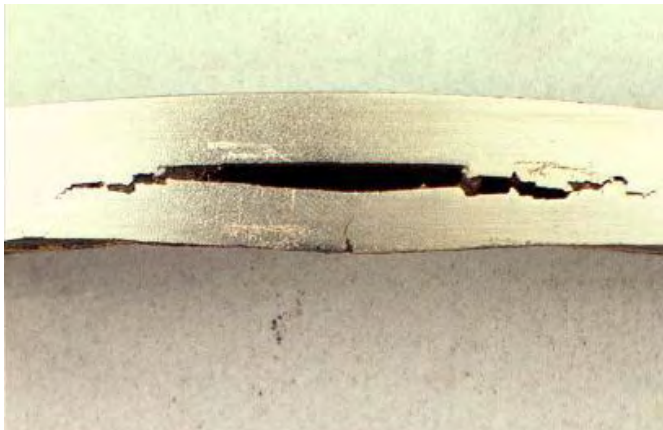
Fig. 4 - Hydrogen Induced Cracking in linepipe steel
